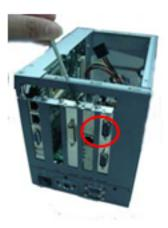
Step 4 Locate the PCI slots from the side.
